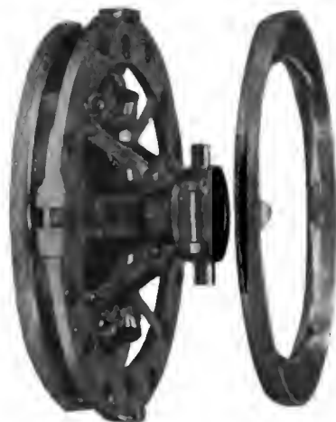
AUTOCAR CLUTCH WITH CORK INSERTS.
